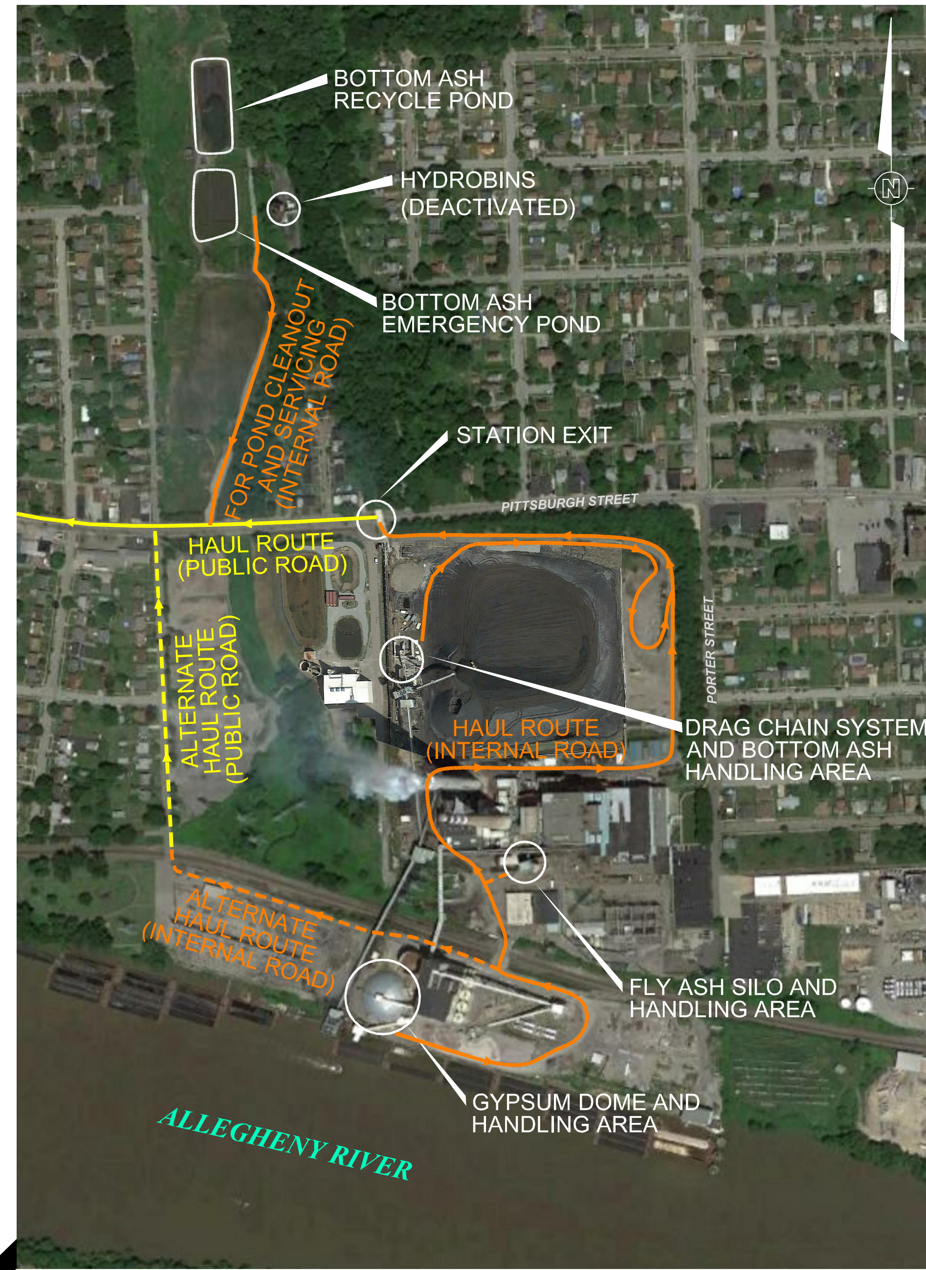
CHESWICK GENERATING STATION PROPER ENLARGED SITE PLAN
